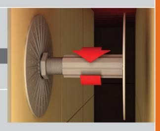
3. Shuttle the locking washer into position.
