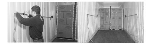
Securing the Freight: Once the remaining freight has been loaded, pull the two pieces of loose 6 banding around the end of the load and use a buckle to fasten the pieces of banding together in the center of the load. Corner protectors may be needed to prevent the banding from damaging the packaging. After buckled, pull tight and then use a banding tensioner to secure the freight.
