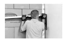
Removal of the LogiTrack: Remove foam inserts from both Pockets. Insert the 2x4 into one Pocket to use as a prybar. Pull 2x4 away from the freight using slow and steady pressure. Continue to pry and pull LogiTrack until entire Track has been removed. Repeat this process for opposite side.
