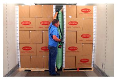
CAUTION - over inflating an air bag may cause freight damage, bodily harm, or cause Logistick loadbar or wedge products to fail. Additionally, when using an Air Bag in conjunction with Logistick loadbar or wedge products, please take measurements after the Air Bag has been installed before cutting your wood.
