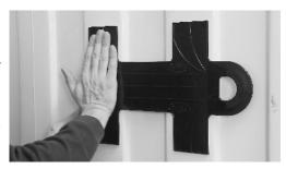
Press firmly against the wings of the Intermodal Strap® to assure that the tape bonds to the wall. Repeat this procedure with the second Intermodal Strap® on the opposite wall, making sure that it's adhered at the same height.
