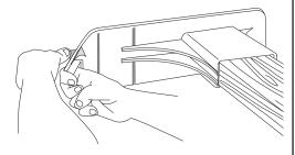
several inches of the adhesive. Next, slowly release the handle and gently secure the exposed portion of adhesive to the trailer wall. Once secure, hold the Loadbar XL® in place with one hand and pull the remaining portion of the backing downward and to the rear of the Loadbar XL®. Make sure the entire tape backing is removed so the adhesive surface is uncovered and exposed to the wall.
