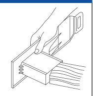
against the cargo. An ample amount of force is needed to slide the second Loadbar XL® into place because of the outward pressure of the system. If the pressure is too great, remove half of ONE foam insert and try to re-install. If the pressure is still too much, remove half of the foam insert from the opposite side and re-install. Never remove all foam from either Loadbar XL®.
